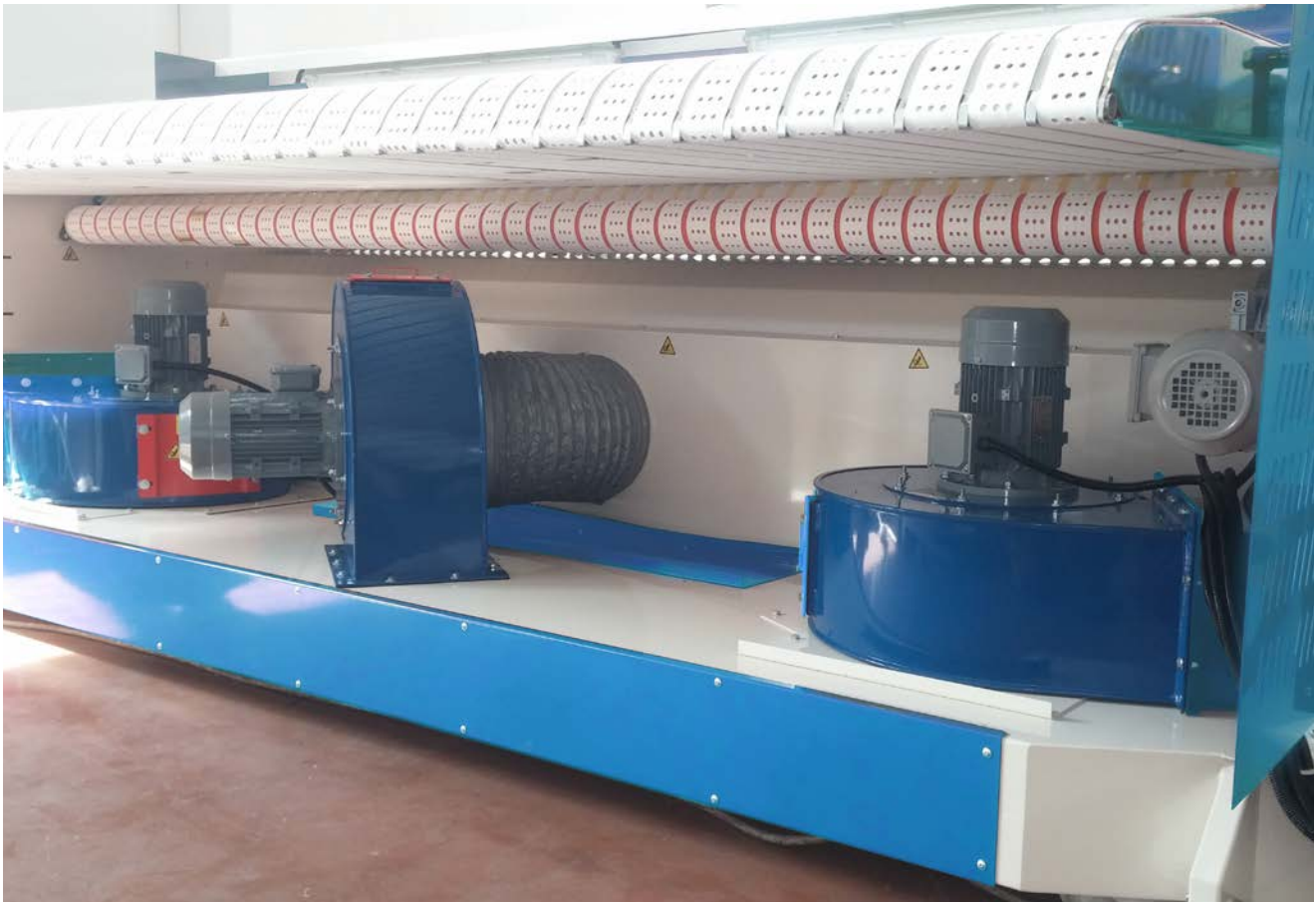
The vacuum conveyor and “Ventomat” chamber efficiently unfold and stretch wet linen
