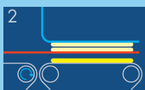
3 The JENSEN bottom-up stacking concept provides compact and very accurate stacking
