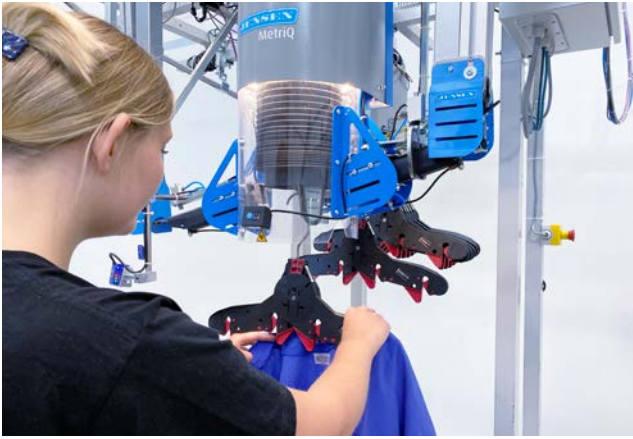
The new position of the hangers enables a silent, stressless operation.
