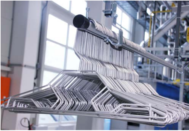
Laundries can run mixed types of hangers on demand, using two inlets at a much higher speed than before.
