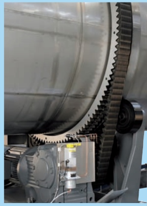
Toothed chain drive with automatic lubrication system
