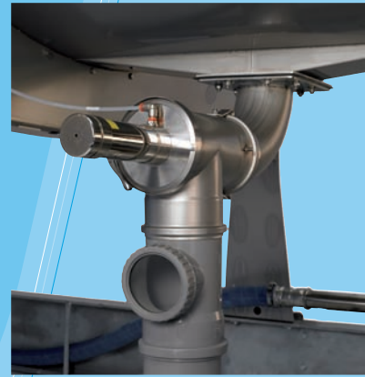
Drain valve with quick-release fixture and sight glass
